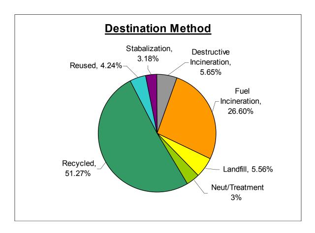
There are two types of incineration: destructive and fuel. The goal of destructive incineration is to simply destroy the material. During fuel incineration, energy is recovered through the burning process and sometimes material will also be recovered.
